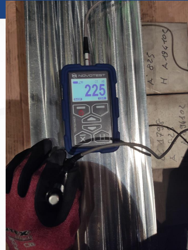
Testing the hardness of welded joints
