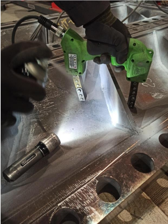
Carrying out magnetic particle testing of welded joints
