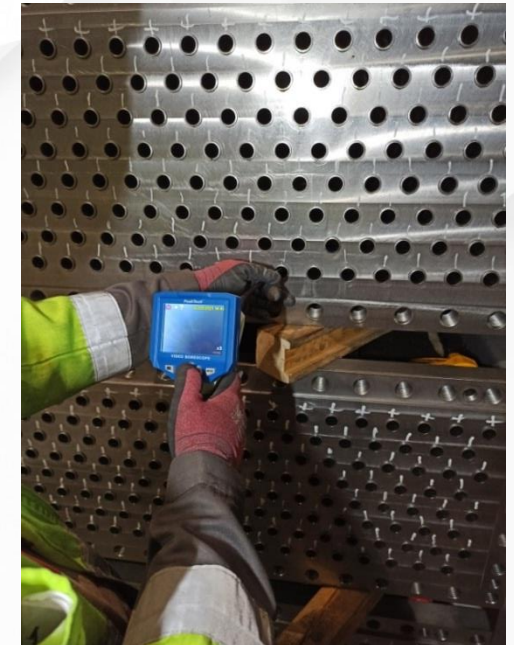
Endoscopic examination of the inside of the tube
