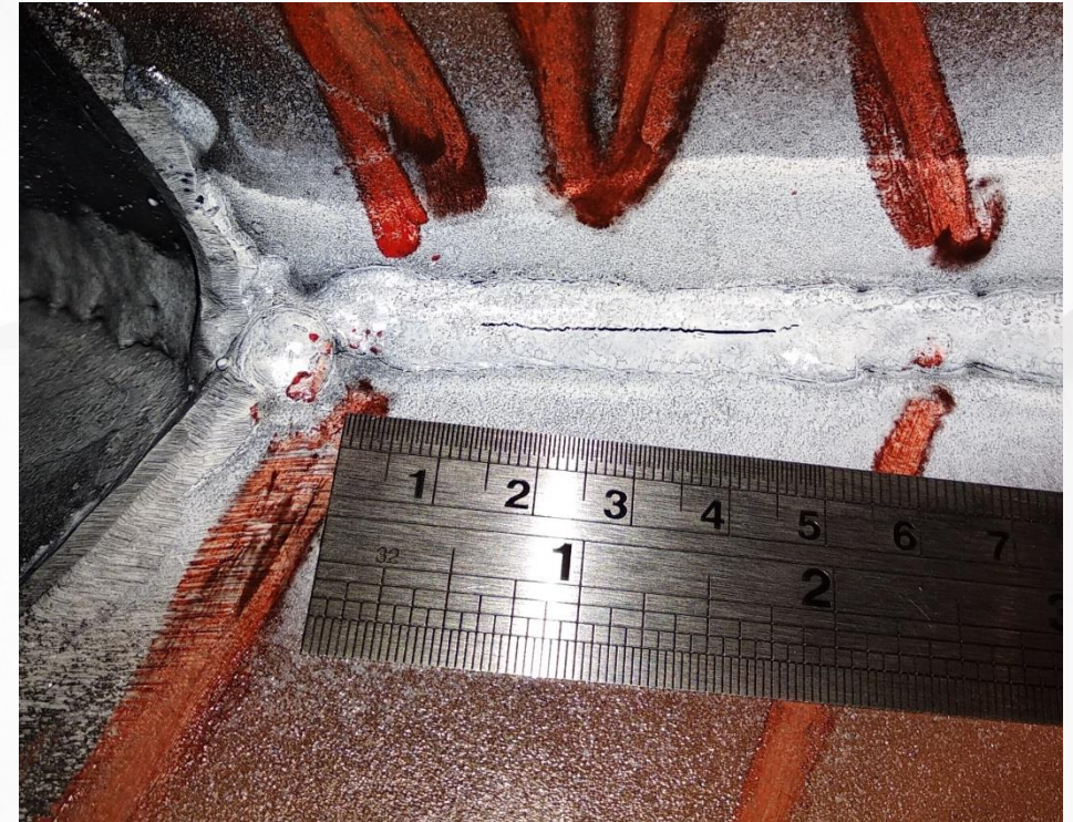
Linear indication in the weld (crack)
