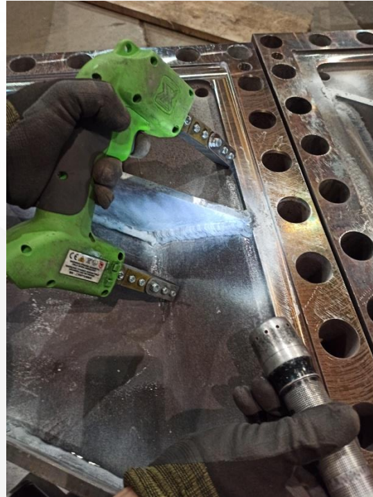
Carrying out magnetic particle testing of welded joints
