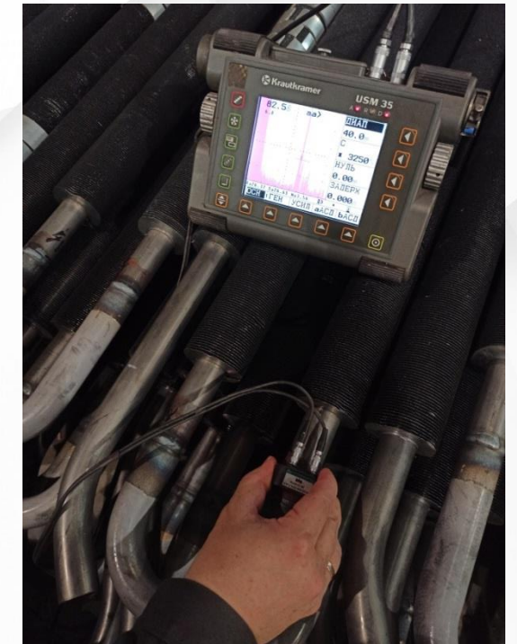
Carrying out ultrasonic testing of welded joints of coil pipes
