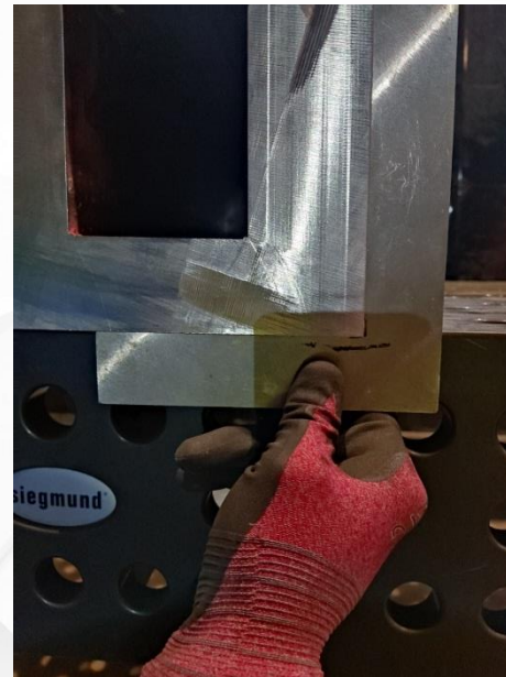
Control by measurement. Checking the perpendicularity of the upper and lower walls
