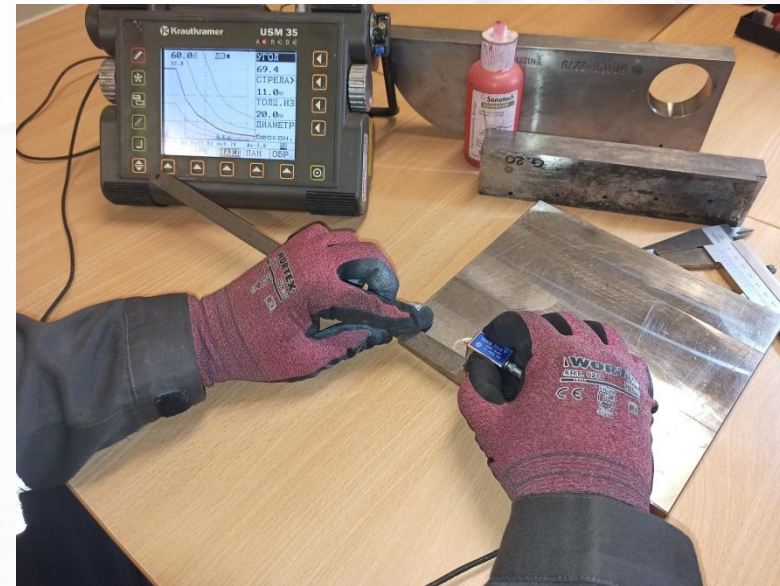
Performing DAC setup for the inspection of welded joints
