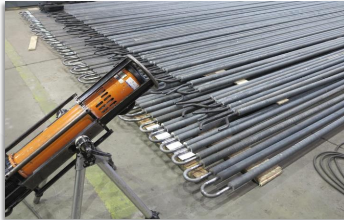
X-ray test of heat-exchange tube welds and U-bends
