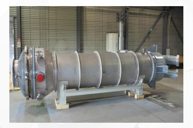
**TMT** has mastered production of heat exchangers,
