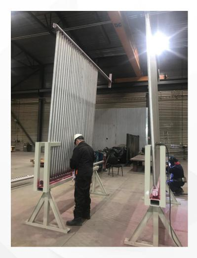
**TMT** has developed and certified welding process suitable for mentioned previously list of steel grades. In this case, production is done with high-performance equipment for **MIG**, **MAG** and **TIG** welding processes (semi-automatic and argon-arc welding).
